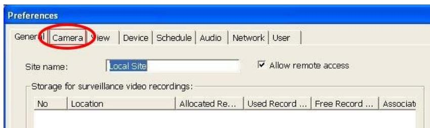
3. Select a Camera button which you want to enable Secure Zone Detection.
