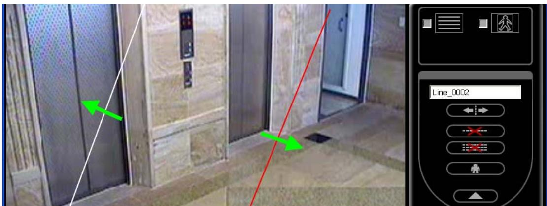
5. For example we draw 2 lines on the video area for Virtual Fence detection.
