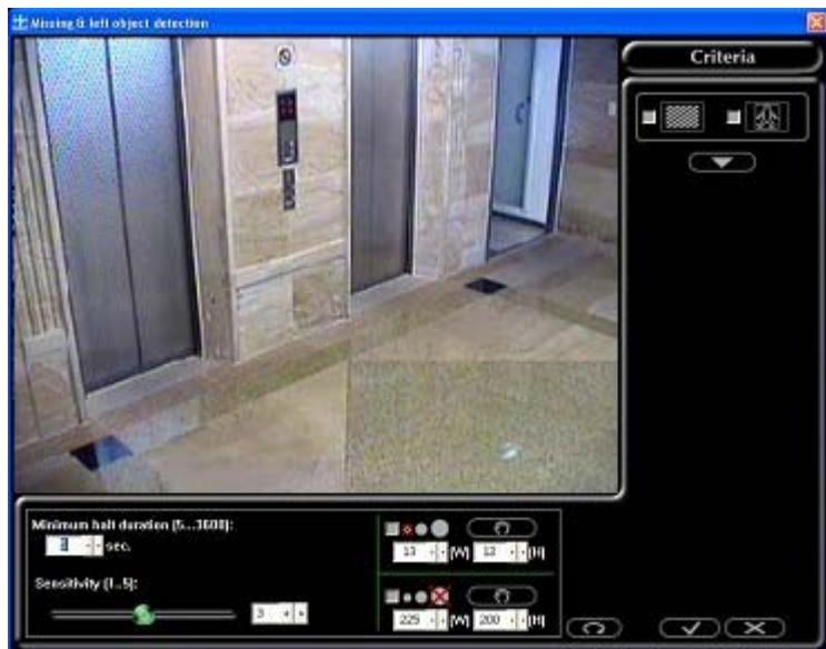
7. The timer to trigger an alarm is shown in the Picture below, and you can change the time in a range of 5~3600 seconds, which is described as **[Minimum halt duration...]**
